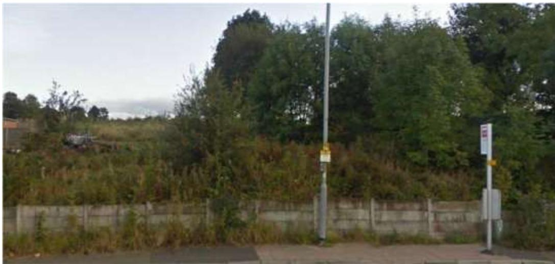
People may have wondered why this land behind the bus stop on the bottom road has never been built on and have been left as no-man's land. The reason for this is that under this plot were the access shafts to Redhouse Colliery Coal Mine. Even though these shafts have long since been filled in they can still be very problematic for developers.
